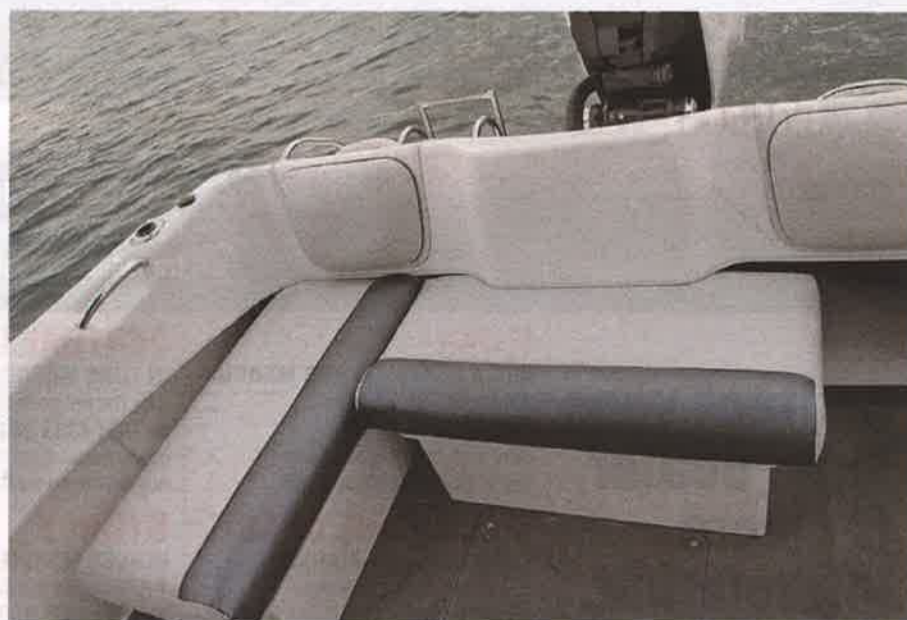
Complete versatility in aft seating allows the padded bins there to be moved into several positions or completely left out of the craft.
