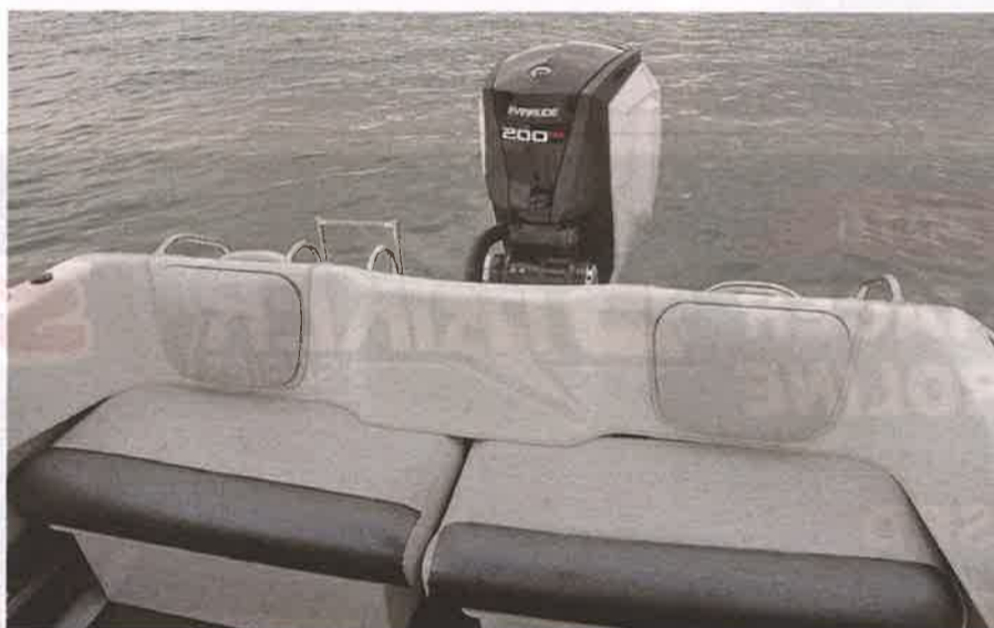
There's seating for three people on padded storage bins at the transom. You can also move the bins around to a different configuration when necessary. The oval backrest sections can be removed to allow boarding from astern.
