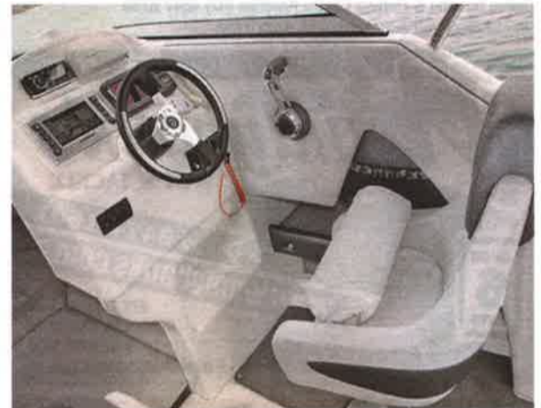
An easy to monitor dash design is highlighted by the premium Evinrude Icon Colour touch gauge linked to the 200 Gen 2 E-Tec plus the Lowrance Elite 7. Other switches for various functions plus the winch are lower, but still within easy reach.
